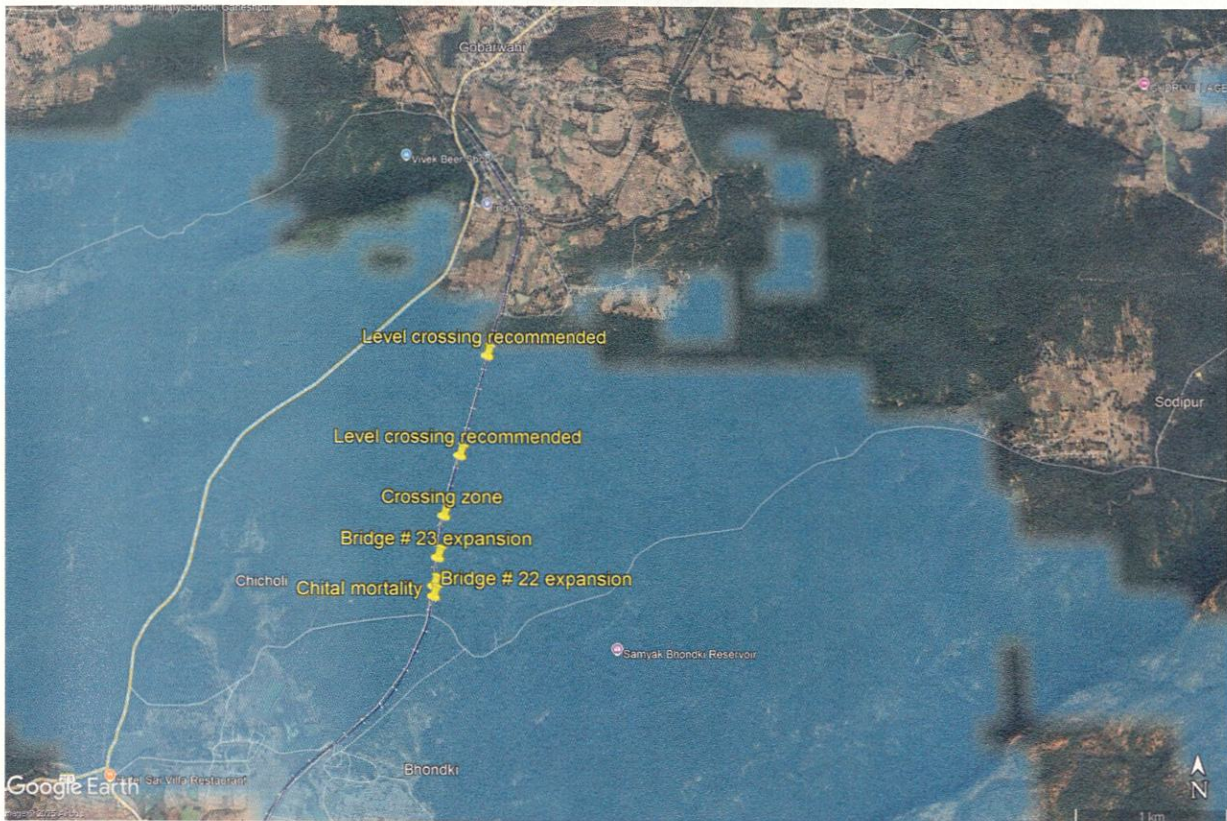
Figure 3.14.13: The Dewhadi-Gobarwahi railway line passing through the forest patch before Gobarwahi. Wildlife movement here is rampant, consequently multiple bridge expansions have been recommended here.
