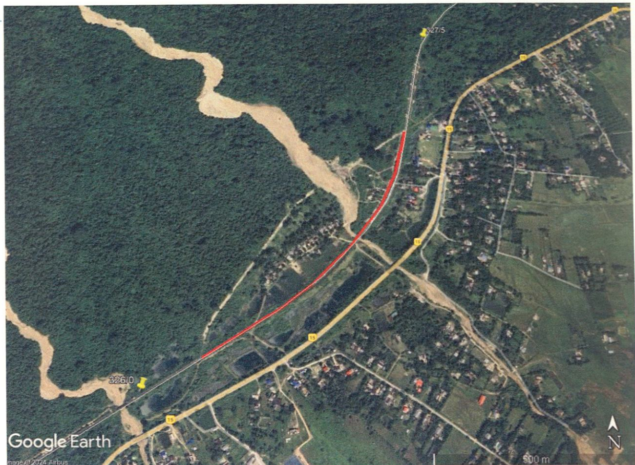
Figure 3.3.6: Approximately 950 m of the railway track (in red) where construction of ramps is not required, and where fencing is to be done to discourage elephant movement into human settlement south-east of Dulung Forest Reserve.
