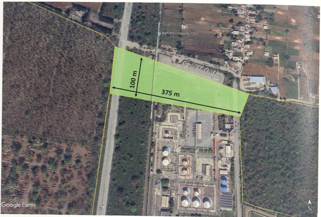
Figure 3.10.7: Suggested location of the wildlife overpass over the NH 109, railway track and IOCL compound (green polygon) and fencing (yellow lines) funnel wildlife movement towards the overpass.
