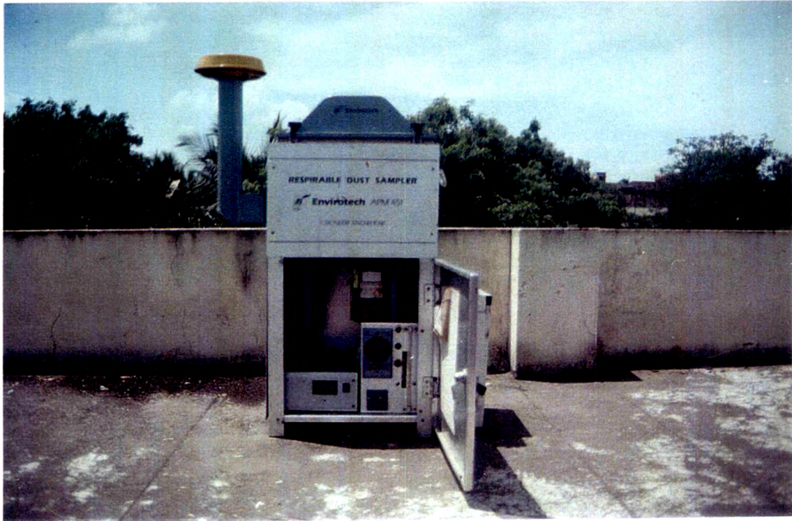
Plate 5 Respirable Dust Sampler (Model. APM 451, fabricated by Envirotech)
