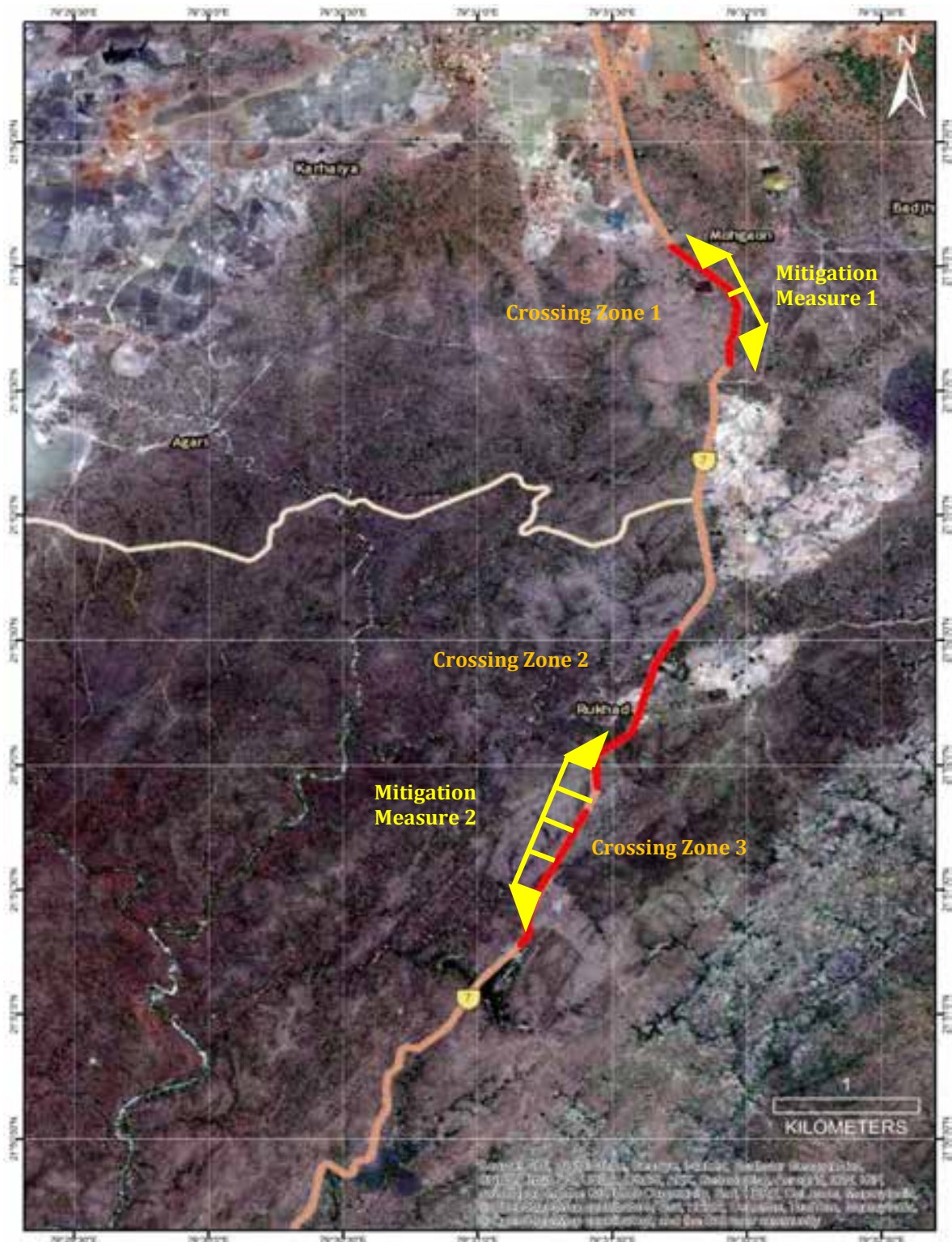
Figure 8: Location of multi-species crossing zones and mitigation measures on NH-7 Patch 1 identified by kernel and overlay analysis based on intensity of signs across the road stretch
