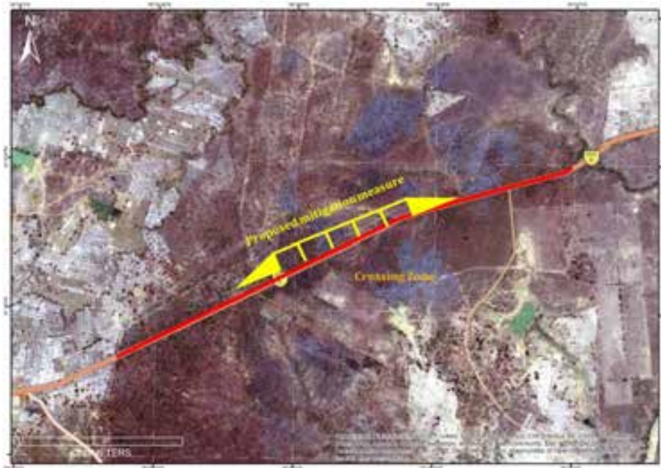
Figure 27: Location of species specific crossing zone on NH-6 Patch 10 (MH) identified by kernel and overlay analysis based on intensity of signs across the road stretch and location of proposed mitigation measures
