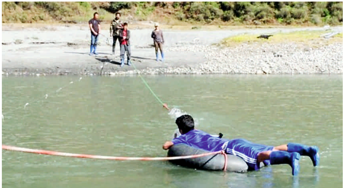
Figure 9.1: Field measurement of velocity and depth at 2-m intervals
