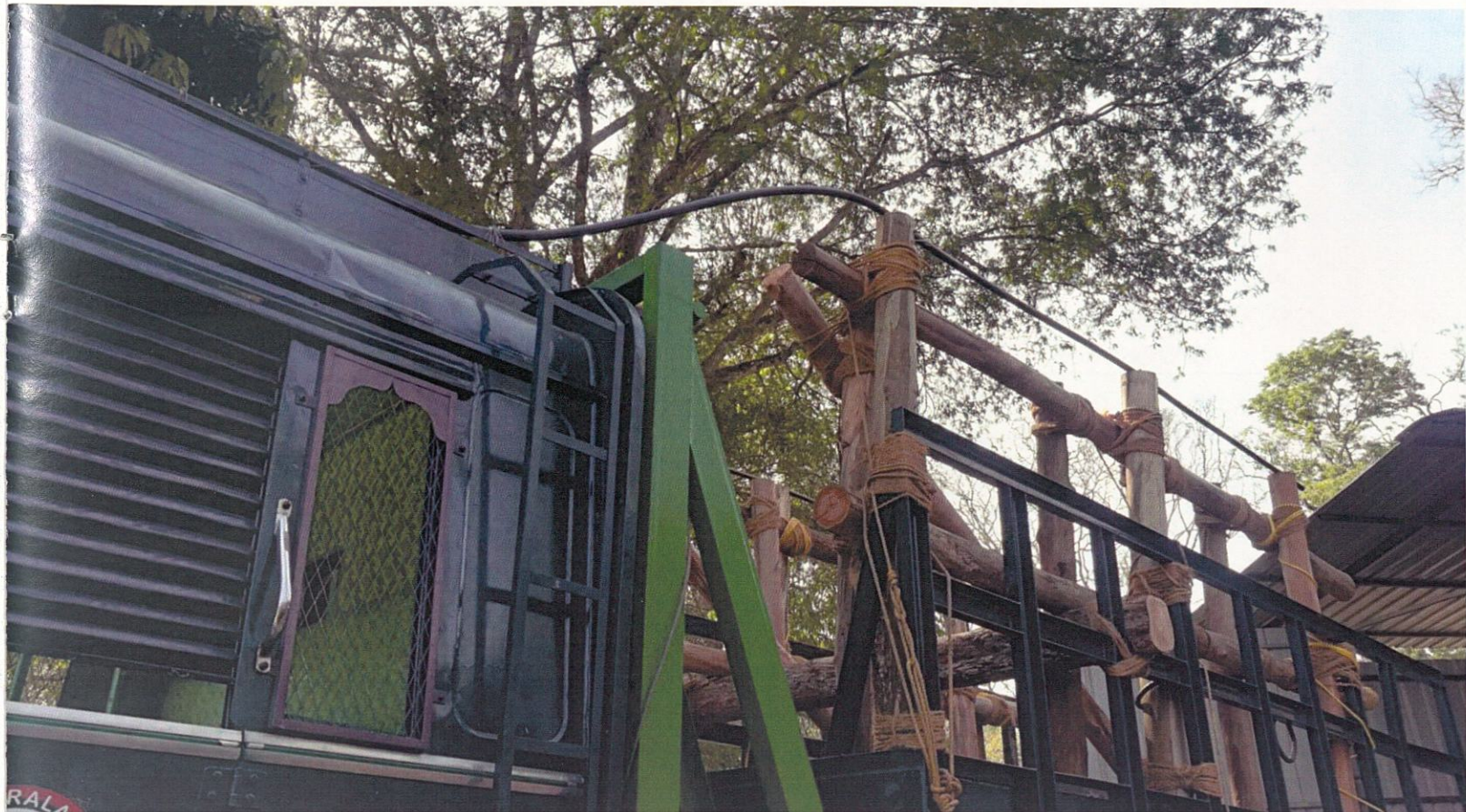
Figure 2b: Kerala Forest and Wildlife Department elephant rescue vehicle prepared for operation. Note the topmost lining with PVC material to negotiate electric lines.
