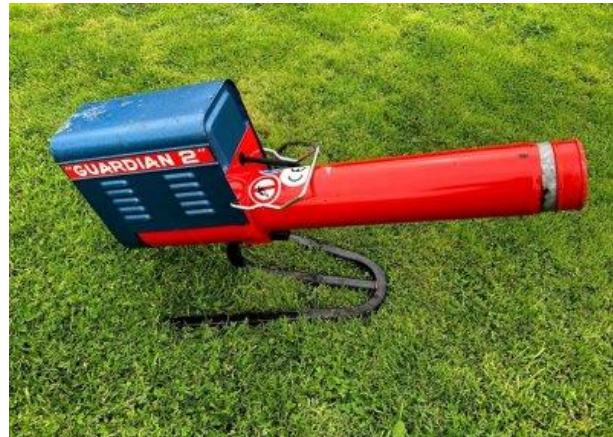
(d). Gas cannons used to scare away birds.
