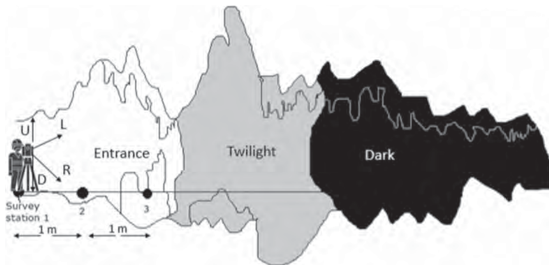
Fig. 2 Illustration of the dummy cave with the survey stations at a one-meter distance, across the caves, beginning from the cave entrance. L left, R right, U up, D down
