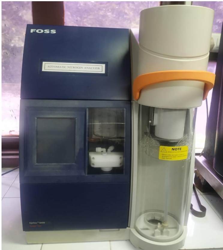
Image 5.7: Kjeldahl apparatus used for the estimation of crude protein of a given sample.
