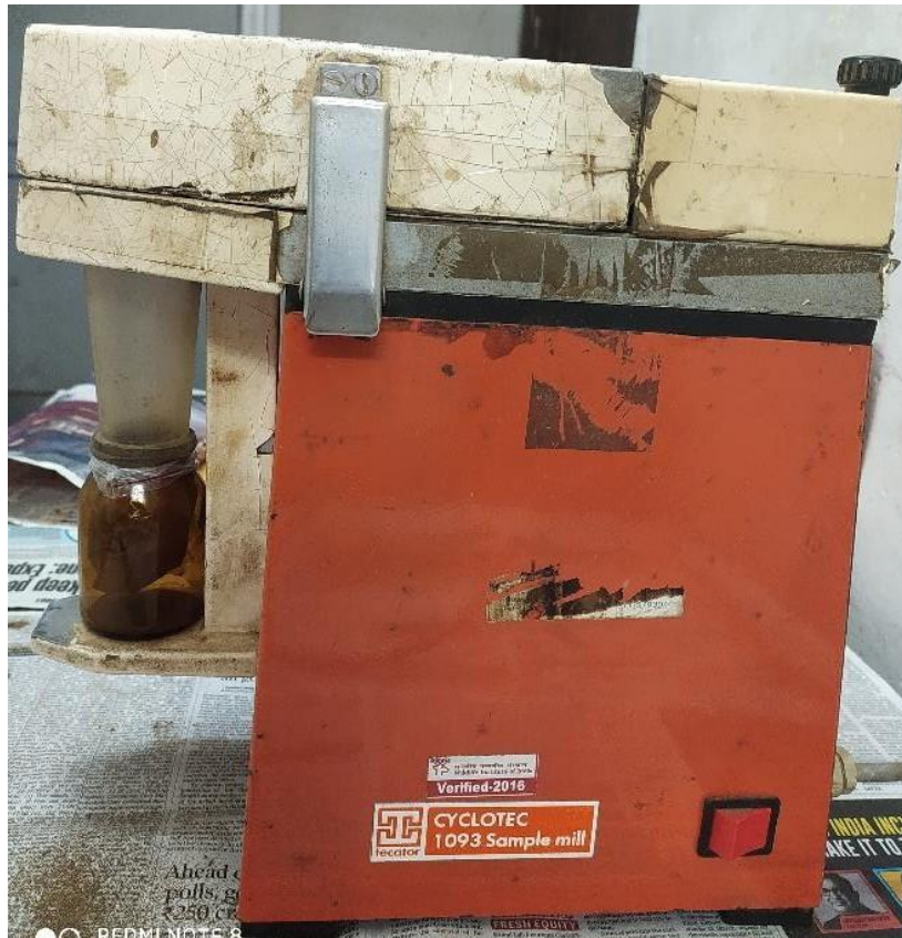
Image 5.1: Cyclotec machine used to grind sample up to 1mm fine powder for the preparation of slides.
