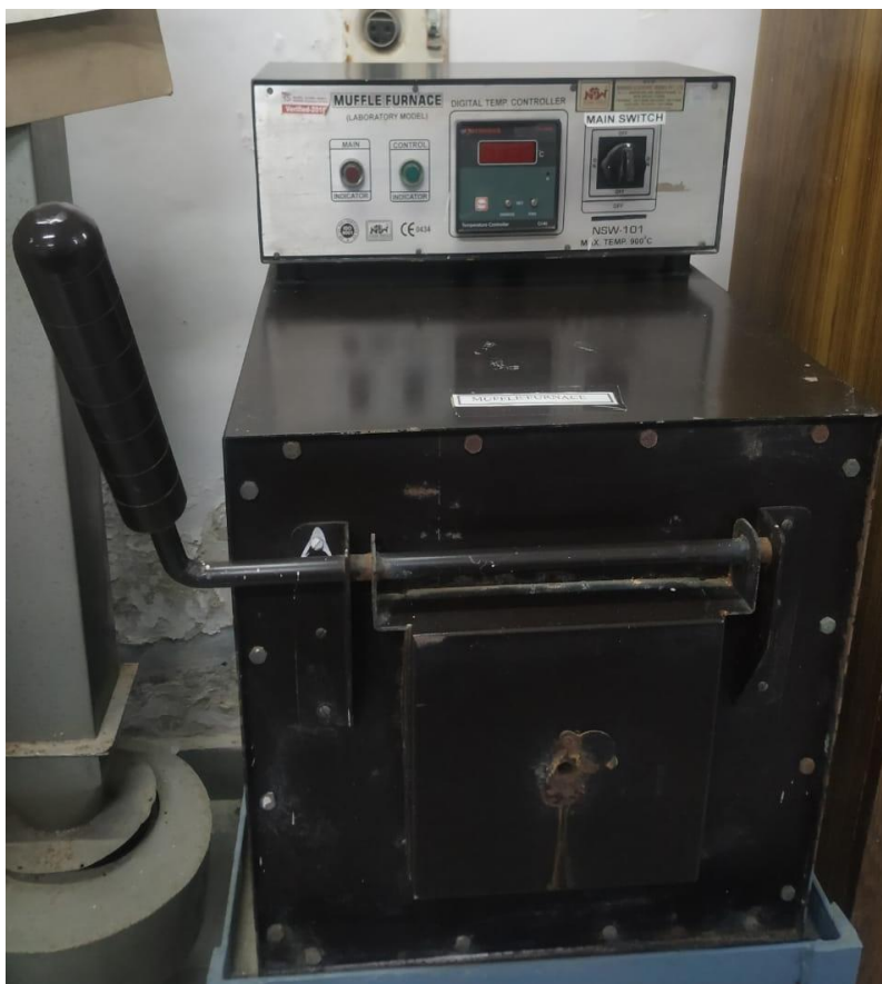
Image 5.8: Muffle Furnace is a unique test cabinet designed to detect the percentage of ash content in a particular test specimen like rubber, elastomers.
