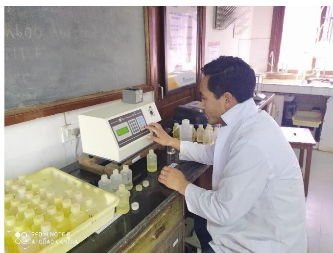
Image 5.6: Estimation of chemical analysis like K and P through Spectrophotometry apparatus.
