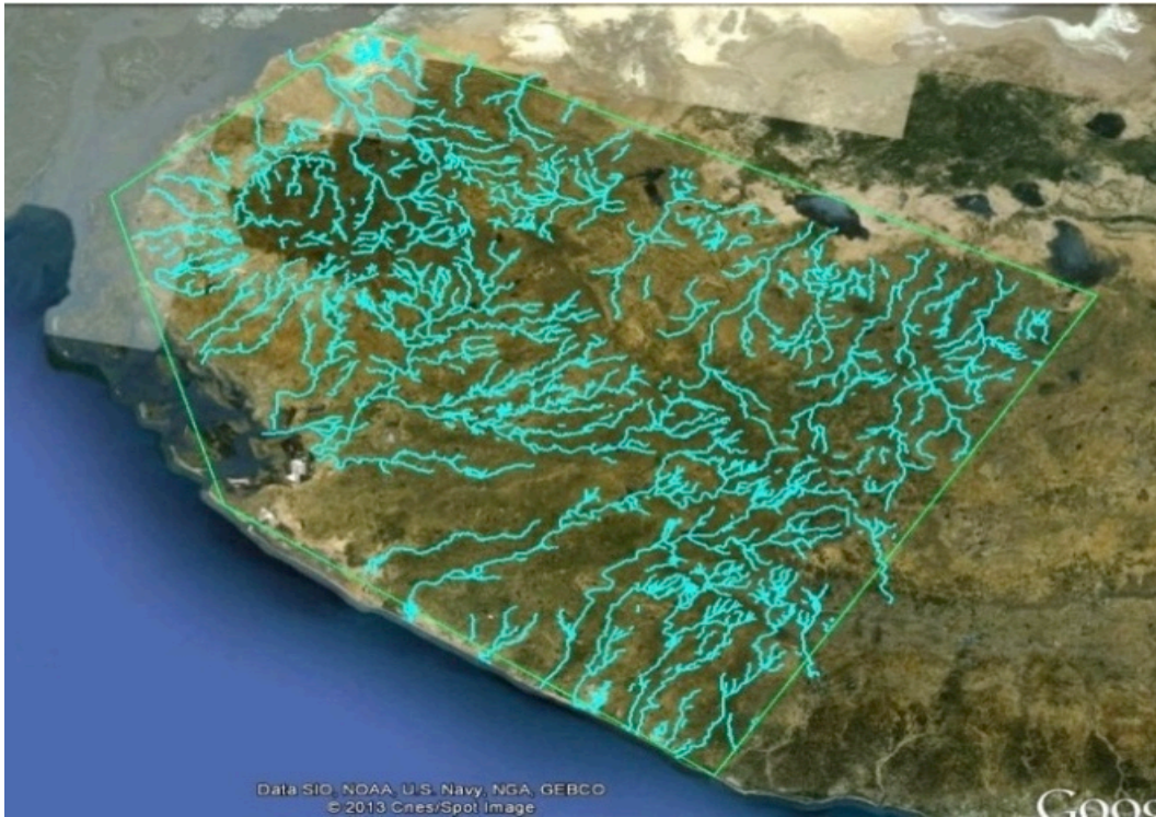
Figure 5-12: Drainage (rivers, streams & gullies) digitized in the study area
