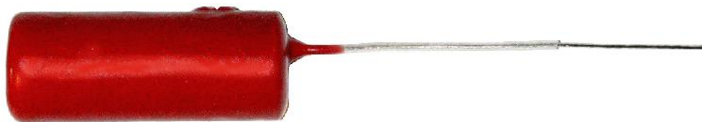
Fig. 2.3. Implantable VHF radio-transmitter (AI-2 Holohill model)
