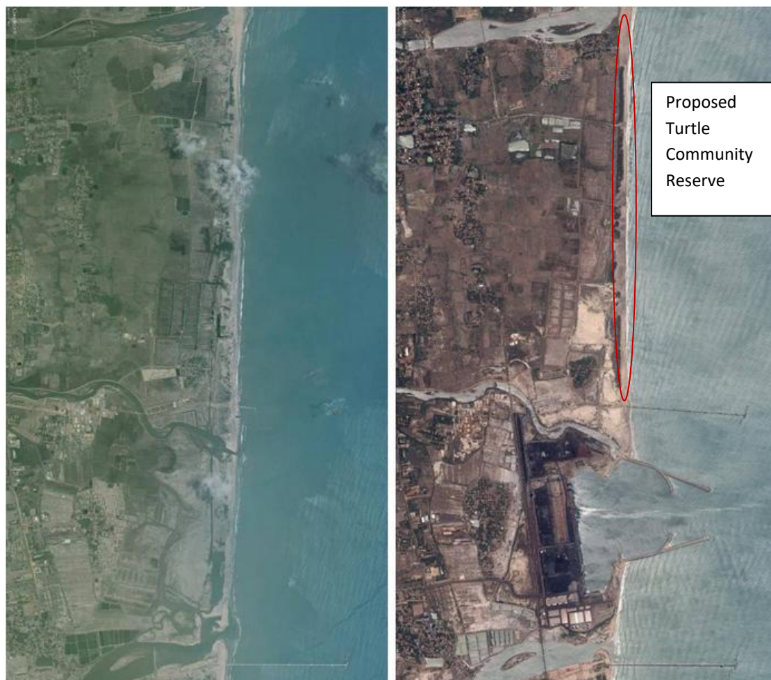
Figure 17 Time stamp images from Google earth of the Karaikal coastline showing changes in the beach morphology along this coast before and after Karaikal port construction. The port is located near to the Vanjur beach
