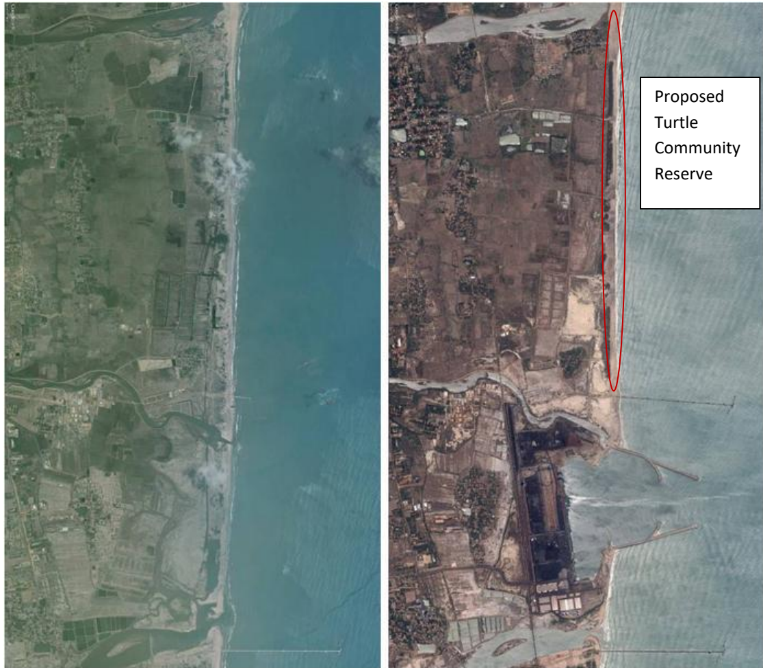
Figure 3.3. Time stamp images from Google earth of the Karaikal coastline showing changes in the beach morphology along this coast before and after Karaikal port construction. The port is located near to the Vanjur beach.
