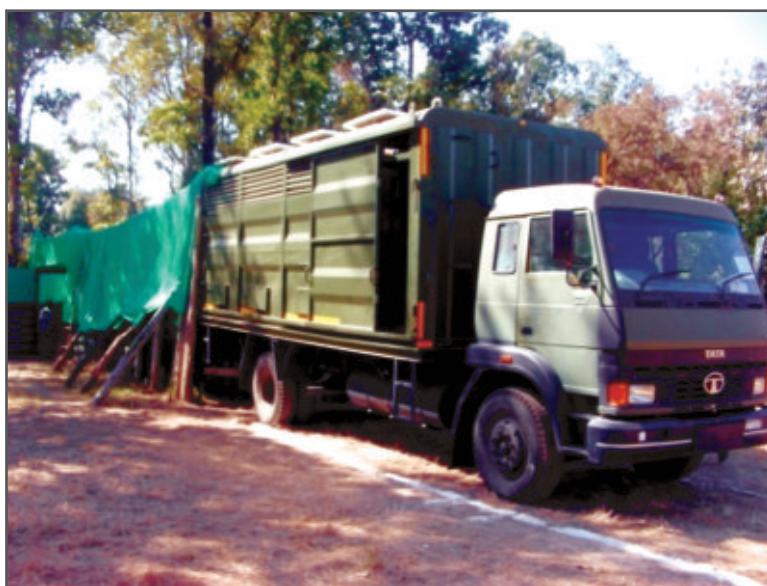
Figure 4: Truck fabricated for transportation of gaurs
