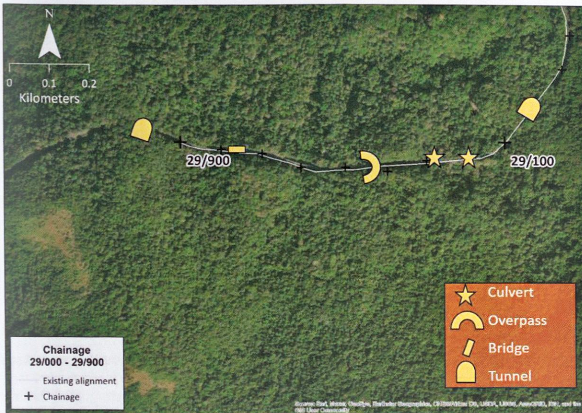
Figure 45: Locations of mitigation measures on chainage 29/000 – 29/900 to be constructed on existing and proposed railway track (NOTE: locations are approximated to the nearest chainage).
