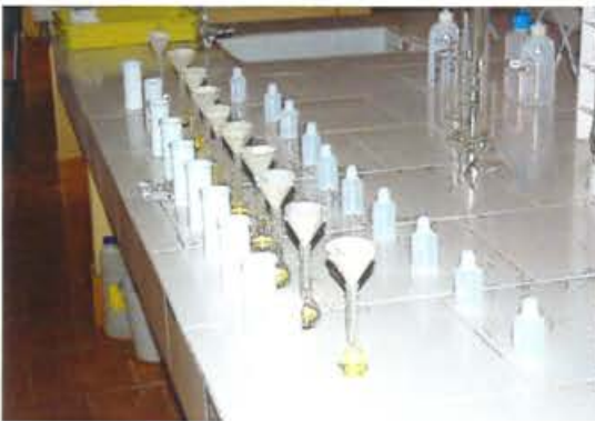
Filtration of digested samples through filter paper
