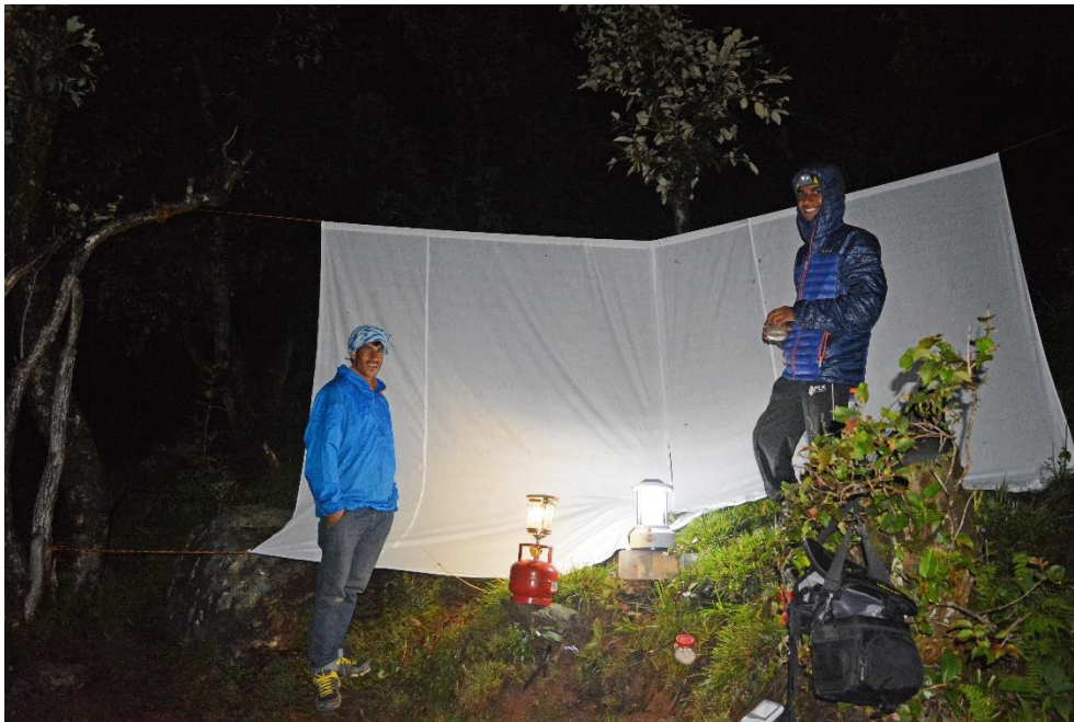
Fig. 2.5: A usual light-trap set up with Solar Powered Lantern and Gas petromax lamp
