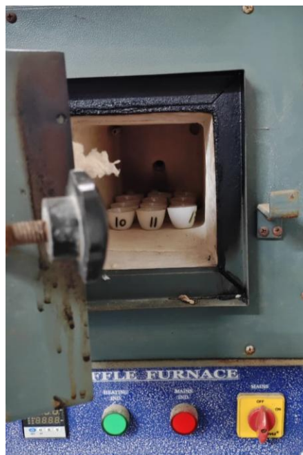
Residue after combustion in muffle furnace for Ash content
