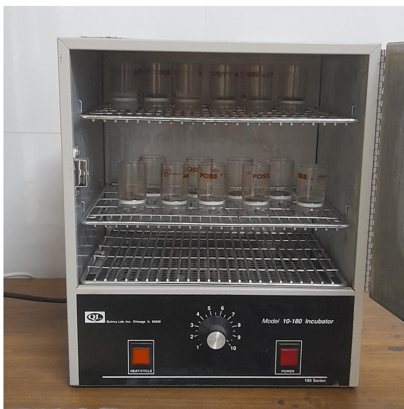
Oven drying samples overnight for ADF estimation
