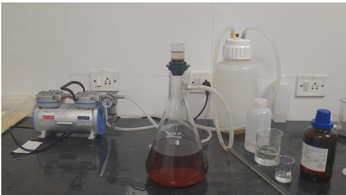
Filtering of refluxed sample using low vacuum for ADF estimation
