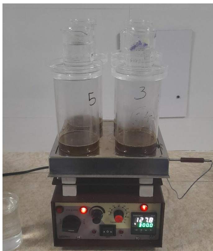
Refluxing of samples in acid detergent solution for ADF estimation
