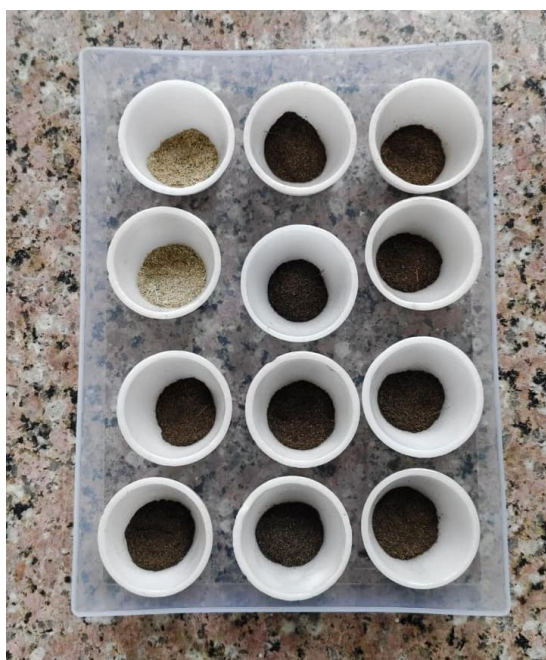
Residue after combustion in muffle furnace for Ash content
