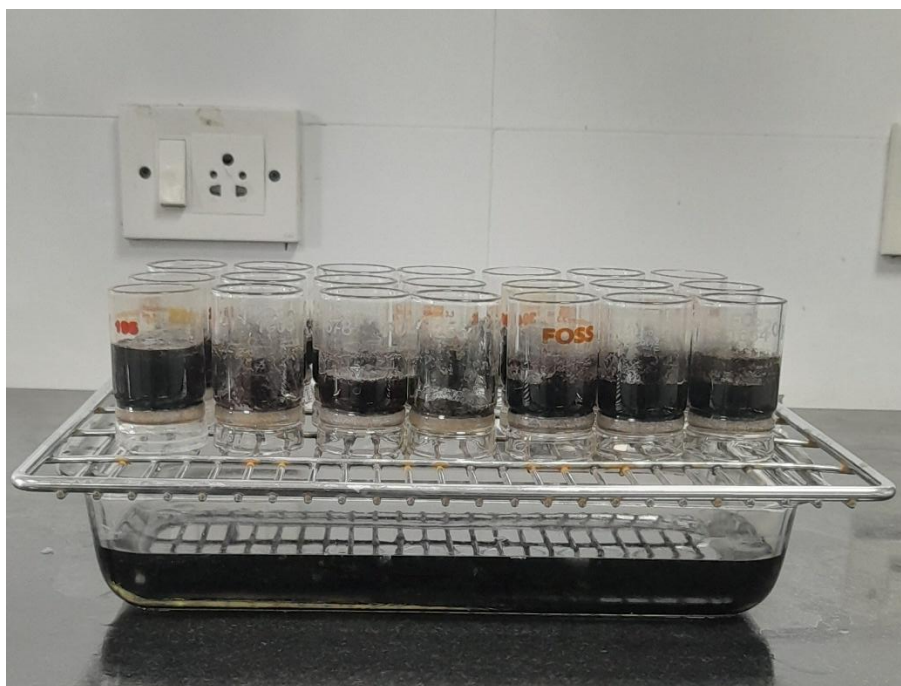
Treating ADF residue with 72% sulphuric acid for ADL estimation
