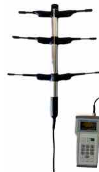
Figure: Tracking Antenna and Radio Receiver
