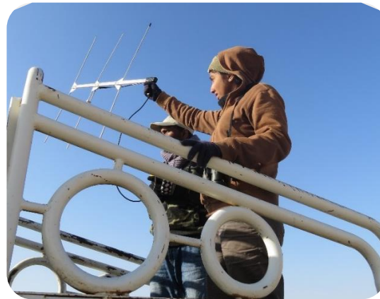
Plate 2. Homing in on one of the radio-collared dogs using a three-element Yagi antenna with a handheld receiver (Habit model HR 2600)
