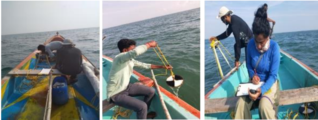
Figure 35. Structure for drop down quadrat with GoPRO fixed on it. B. Assessing the transparency using a Secchi Disk. C. Dropping of the quadrat
