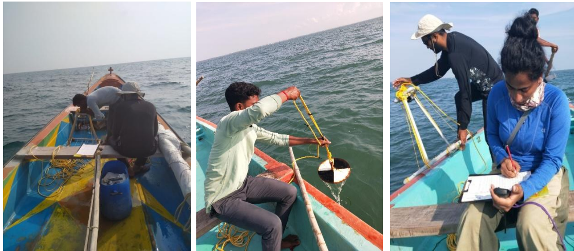
Plate 2.3.: A. Structure for drop-down quadrat with a GoPro fixed over it. B. Assessing the transparency using a Secchi Disk. C. Dropping off the quadrat and recording the observation. Photos credits: Sweta Iyer, Sohom Seal, Ajith Kumar.
