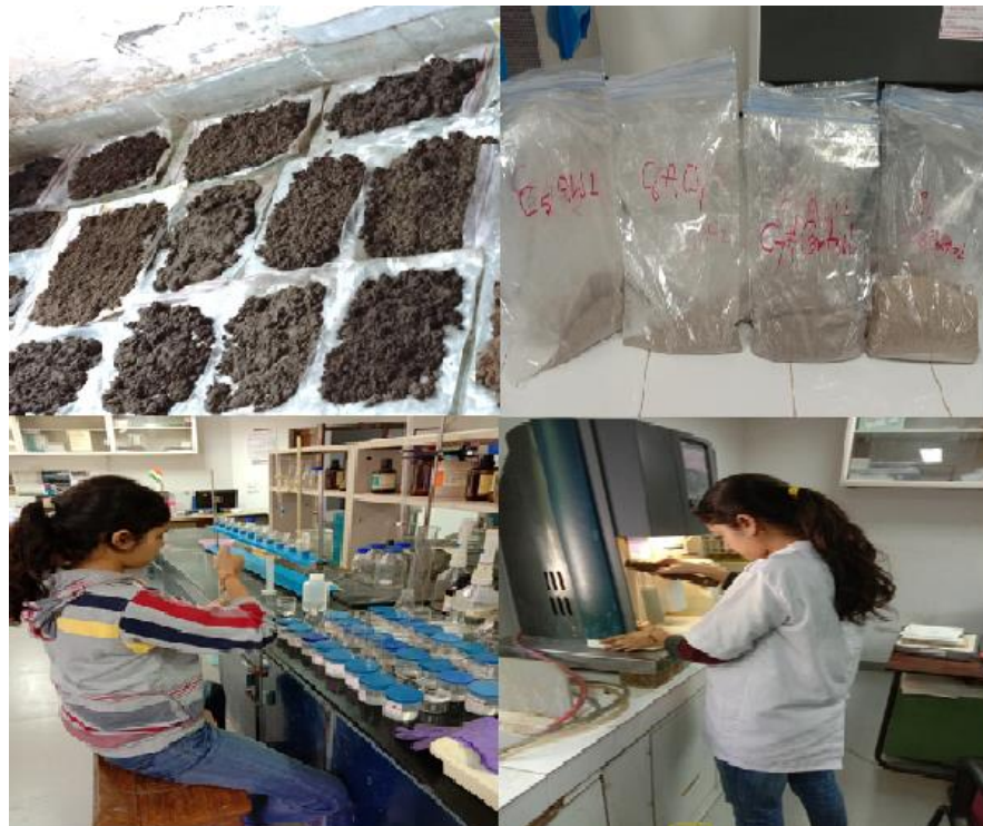
Figure 5.7: Air drying and preparation of sediment and seagrass samples for nutrient analysis at WII laboratory
