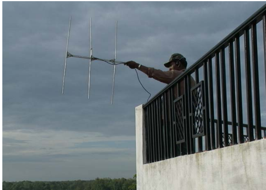
Plate 4. Tracking of radio-collared dhole with the help of a VHF receiver and Yagi antenna from a vantage point in Pench Tiger Reserve, Madhya Pradesh.
